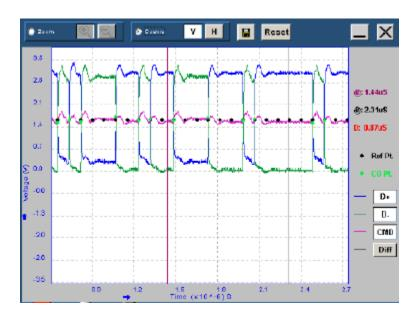
Select the Horizontal cursors to change the positions, and read the voltage values on the Y-axis.
