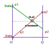
The intersection of the four voltage points p1, p2, q1, and q2 gives the Cross-Over point for Voltage level (y) and time (x). x and y coordinates are obtained by solving the following two equations:
