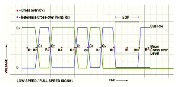
The following figure explains the interpolation technique used to find the actual cross over where p1 and p2 are the adjacent data points after q2:
