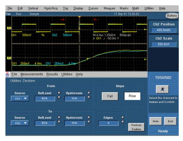
19. The zoomed section of the waveform available on the lower part of the screen shows the results of the deskew operation clearly. You will see that after performing the deskew operation, the skew is automatically removed.
